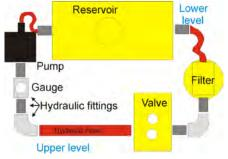
Figure 5: Hydraulic layout seal surrounding
