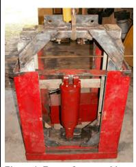
pair of 6" long pieces of light angle-iron were welded on the underside of the top lintel to hold the upper die blocks. A heavy block with an appropriate hole for the pin for the lower end of the cylinder was welded to the lower lintel. Figure 4 shows that arrangement as well as the partially constructed cabinet.
